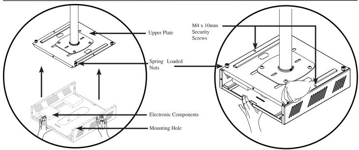
**Step 6.** Lift the equipment tray into position.
